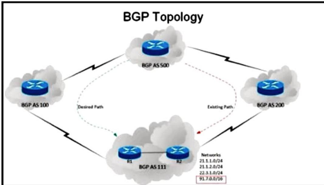
An engineer has been asked to redesign the traffic flow toward AS 111 coming from AS 500. Traffic destined to AS 111 network 91 7 0.0/16 should come in via AS 100. while traffic destined to all other networks in AS 111 should continue to use the existing path.
