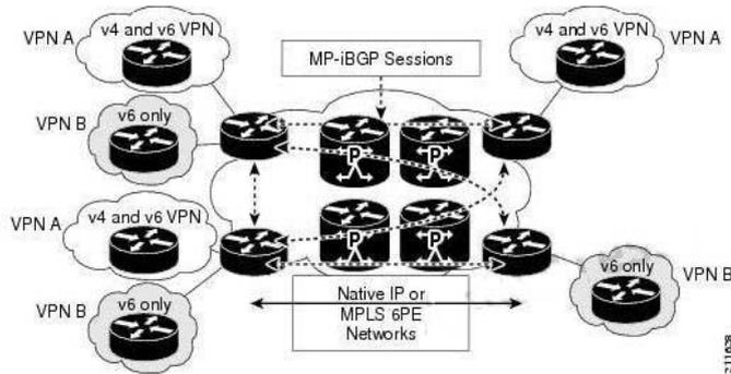
IPv6 VPN service is exactly the same as MPLS VPN for IPv4. 6VPE offers the same architectural features as MPLS VPN for IPv4. It offers IPv6 VPN and uses the same components, such as:
