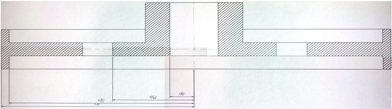
This section view was dimensioned using Baseline Dimensions. The dimensions are too close together which impacts the drawing's legibility.
