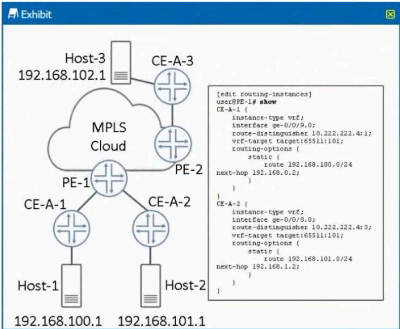
Referring to the exhibit, there is an Layer 3 VPN setup that connects sites CE-A-1, CE-A-2 and CE-A-3 together. Host-1 can communicate with Host-3, but Host-1 cannot communicate with Host-2. What must you do to solve the problem?
