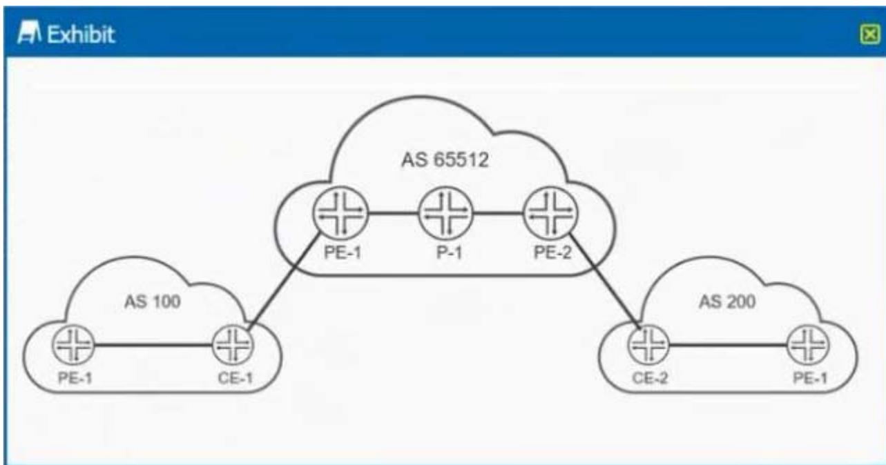
You are providing carrier-of-carrier VPN services for AS 100 and AS 200. You want to distribute MPLS labels between your PE routers and the AS 100 and AS 200 CE routers.
